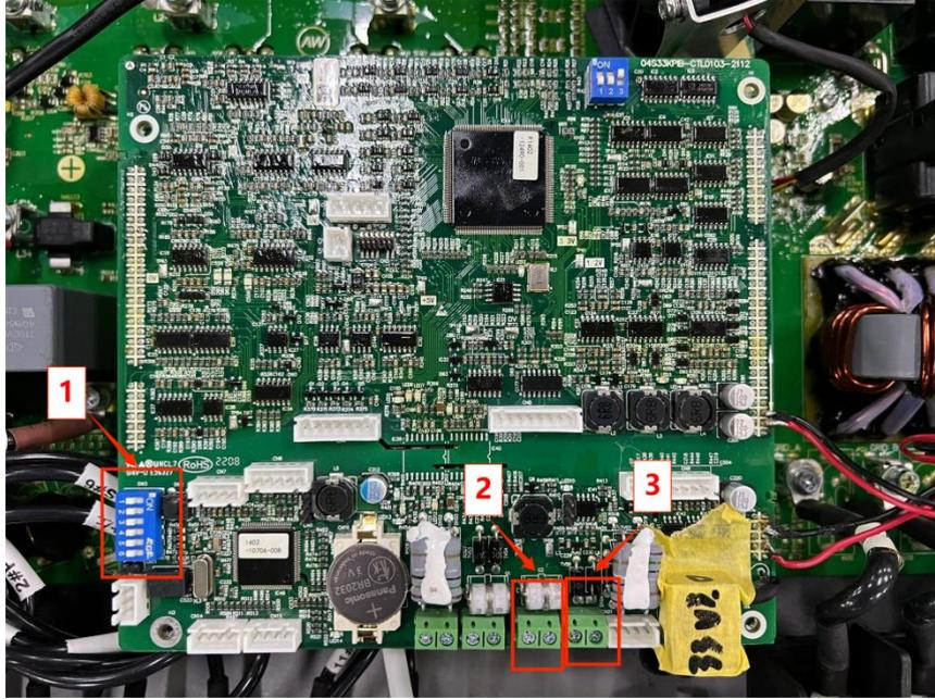
Figure 5-1 Example dip switch on communication board(X2 Series)
