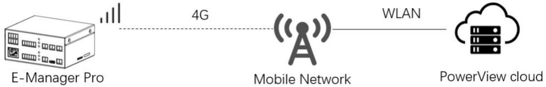
Figure 4-7 4G connection diagram
