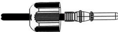
Figure3-17 Crimp the negative metal terminal
