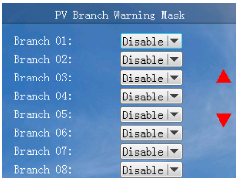
Figure4-43 PV branch warning mask interface
