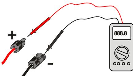
Measure the voltage of PV string < 1000V
