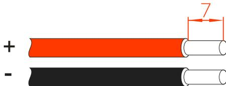
Figure3-32 Stripping diagram of DC input (unit: mm)
