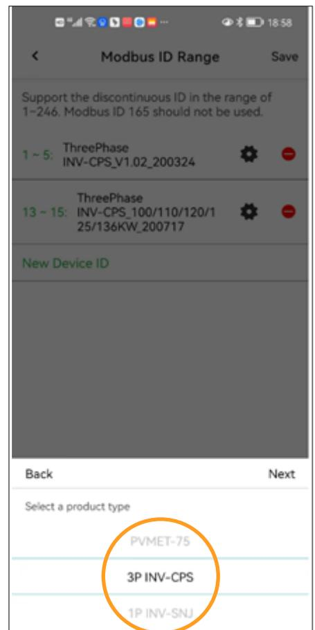
Completely different hardware can be connected on a single RS485 port, requiring the selection of the correct Modbus ID and protocol.
