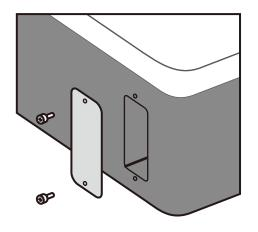
Remove the cover on the slot of inverter.
