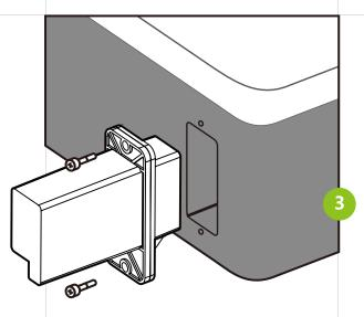
Plug the gateway into the device slot.
