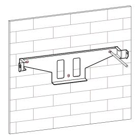
Figure 3-10 Mark the drilling position
