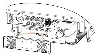
Figure 6-2 Disconnect the connector
