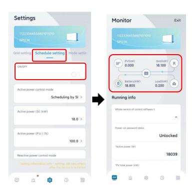
Figure4-13 Battery power-on setting
