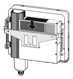
Figure 3-13 Hang the inverter to installation holder
