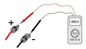
Figure 3-22 Measuring the open-circuit voltage
