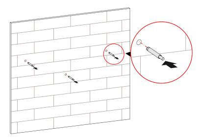
Figure 3-11 Install expansion bolts
