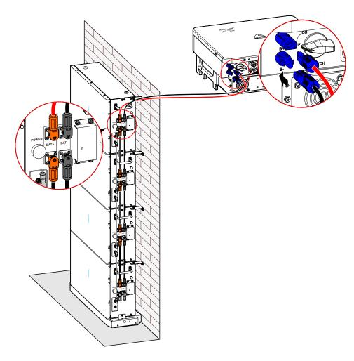
Figure 3-38 Battery wires connection
