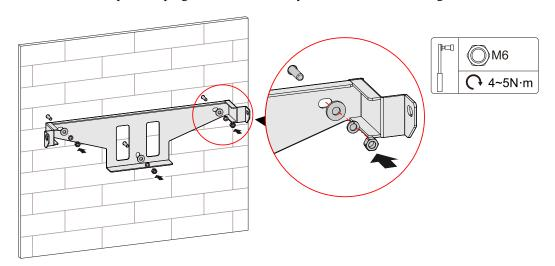
Figure 3-12 Fasten the installation holder
