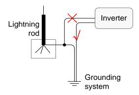
Figure 3-17 The grounding of inverter
