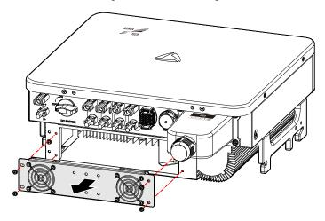
Figure6-1 Dismantle the cover plate
