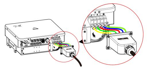
Figure 3-26 Connect the AC output wire
