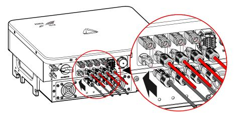
Figure 3-23 Connect PV connectors
