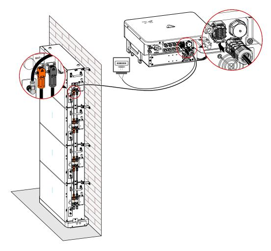
Figure 3-33 COM. communication wire connection
