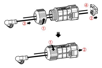
Figure 3-32 Prepare the COM. communication wire
