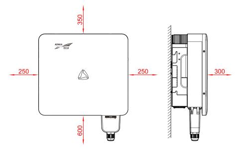
Figure 3-3 Installation clearance (unit: mm)
