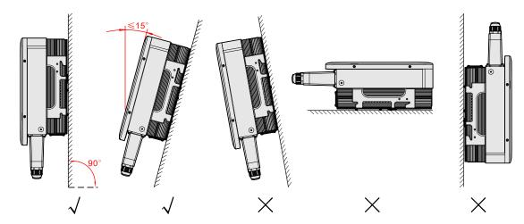
Figure 3-4 Installation method
