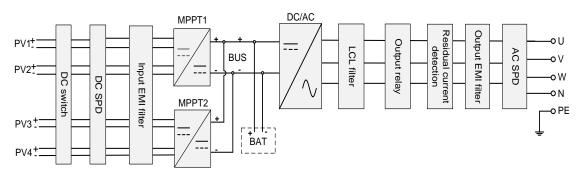
Figure 2-6 Working principle diagram
