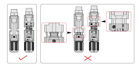
Figure 3-24 PV connector installation method
