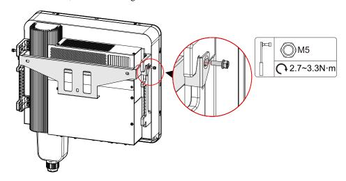
Figure 3-14 Fasten the inverter
