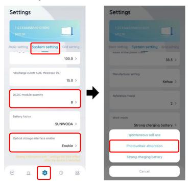
Figure 4-12 DCDC module quantity and work mode setting
