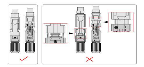
Figure 3-39 Energy storage connector installation method
