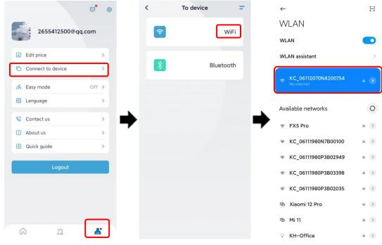
Figure4-9 Connect device
