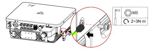
Figure 3-16 External grounding connection
