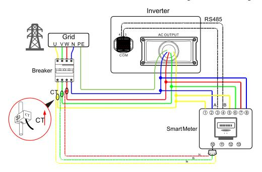
Figure 3-31 Connection diagram between smart meter and inverter and grid
