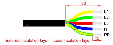
Figure 3-25 Strip the AC output wire (unit: mm)
