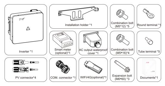
Figure 3-5 Packing list of the inverter
