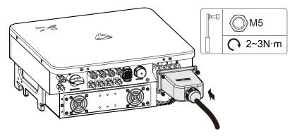
Figure 3-27 Fasten the AC output waterproof cover
