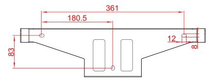
Figure 3-9 Installation size (unit: mm)
