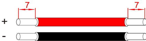
Figure3-34 Strip the battery wires (unit: mm)
