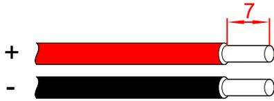
Figure3-18 Strip the PV string input wires (unit: mm)
