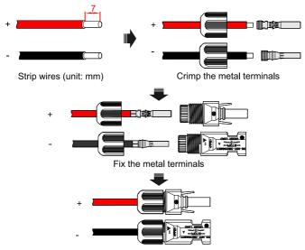
Tighten the lock nut
