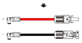
Tighten the lock nut
