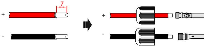
Strip wires (unit: mm)
