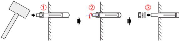
**Step5** Install the installation holder to wall.
