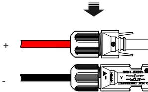
Tighten the lock nut
