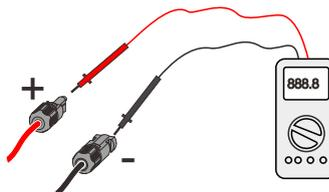
Measure the open-circuit voltage of PV string < 1100V
