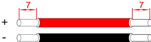
Figure3-34 Strip the battery wires (unit: mm)
